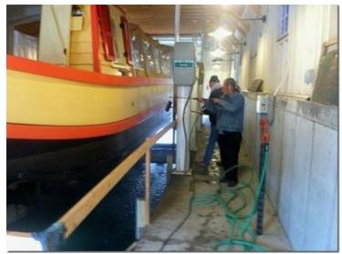
Power washing takes off grime from the black coated aluminum hull. The brightly colored upper part that is above the waterline is made of wood. The boat will stay in its protected canal level building but up on its lift until late April next year.
