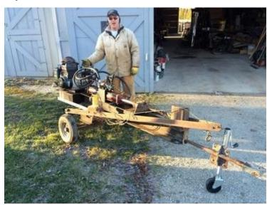
A strange looking new beast is something the MWF crew built in the midst of the cold winter inside the barn. Here Dave Smith prepares to start the gas motor to try out the hydraulic log splitter made from bits and pieces of iron and machinery laying around onsite. This crew is pretty crafty and very
