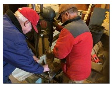
The ShopSmith already put to work by Tom Peters and Brice Crowel as they use the "drill press" feature of this versatile gift. They are drilling deep holes in wooden replicated parts being made to carry the Railway Express Baggage Carts that the M-W-F crew is assembling.
