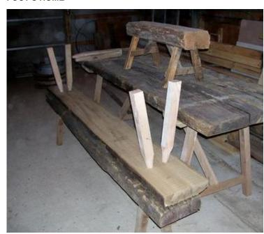
For the interior of the Fouts home, we made benches out of the surplus wood from the huge timbers we received last summer. The sawmill cut two inch planking off the timbers for the seats.
