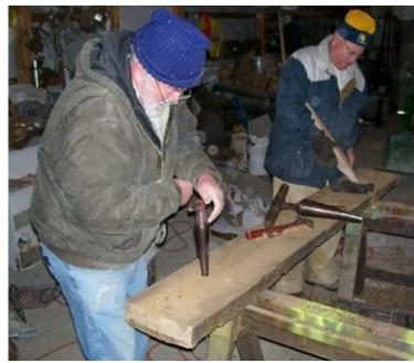
Al Auffart and Vern Cripe use old tools to make the legs for the benches. Later, the upper surface of these historic timbers will be "beat" clean with a rotary nylon power tool before polyurethane sealer is applied, giving them an "old" look that can still be maintained for clean seating.
